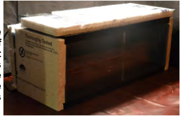
Adding insulation to the top of the Test-1 configuration blocked most of the light from entering the aquarium.
