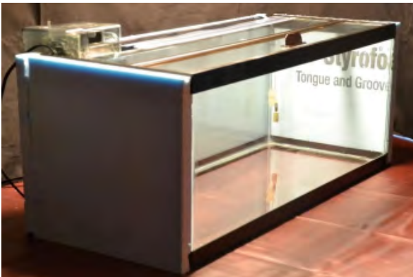
The extruded polystyrene material was more durable and performed better than the other materials used.
