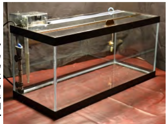
The 20 long test aquarium included a glass top, a HOB power filter, a bubbler and a heater. Shown here without the sand, water or fish.
